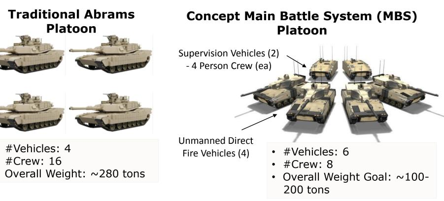
Overall weight savings and crew reduction goal through assignment of traditional functions to unmanned platforms
