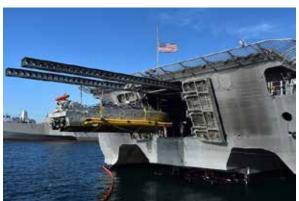
Figure 1: UISS in LCS Launch & Recovery System
