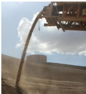
Rocks containing rare earth elements are crushed into pebbles at the Mountain Pass mine in California.
