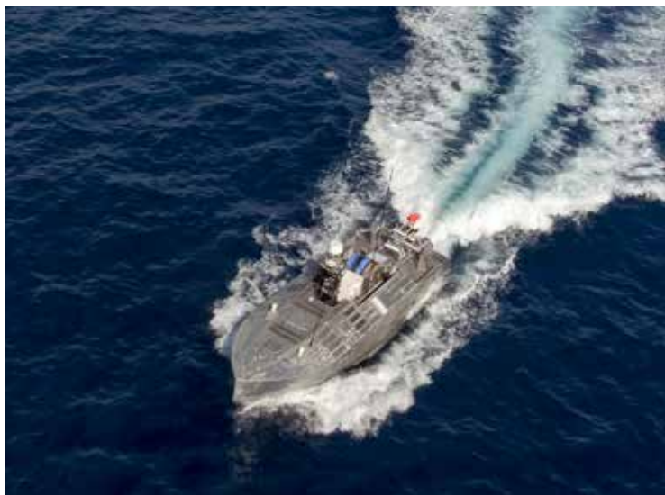
Unmanned Influence Sweep System (UISS) integrated in the MCM Unmanned Surface Vehicle (USV).
