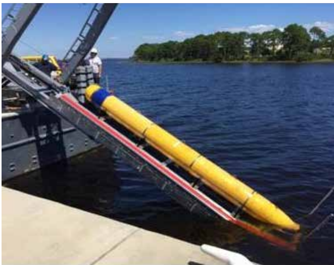
Knifefish UUV detects, classifies, and identifies volume, proud, and buried mines in high-clutter underwater environments.
