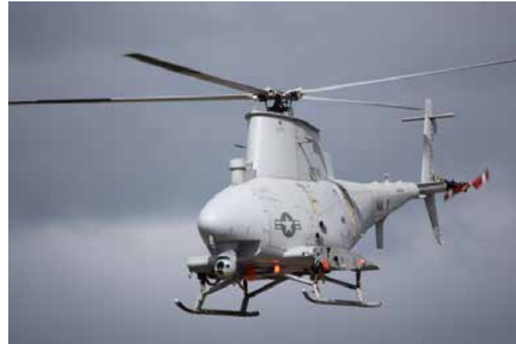
The Coastal Battlefield Reconnaissance and Analysis (COBRA) System, mounted on the nose of an MQ-8B Fire Scout vertical takeoff and landing unmanned aerial vehicle
