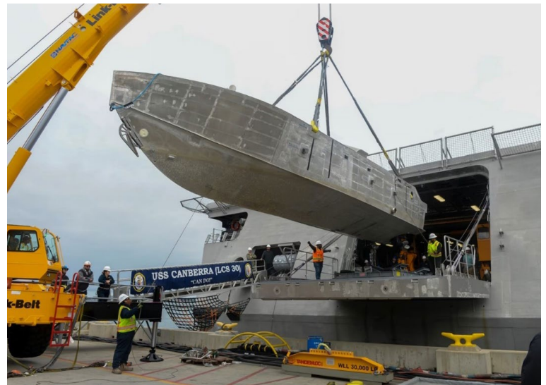
An unmanned surface vehicle is craned aboard the Independence-variant littoral combat ship USS Canberra (LCS 30), as a part of the first embarkation of the Mine Countermeasures (MCM) mission package, April 23, 2024. (U.S. Navy photo by Mass Communication Specialist 1st Class Vance Hand)
