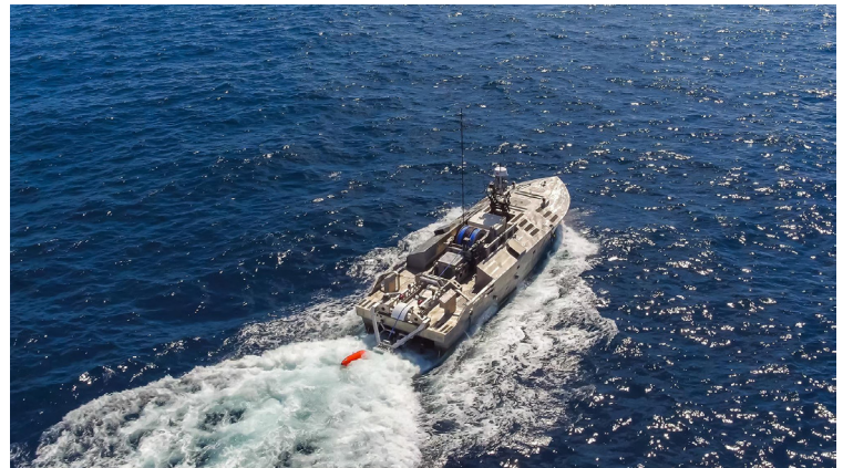
The Unmanned Influence Sweep System is an unmanned, self-propelled, semi-autonomous surface vehicle equipped with capability to sweep acoustically and/or magnetically actuated naval mines. US Navy picture.
