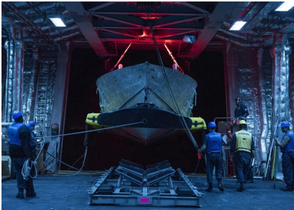
The MCM Unmanned Surface Vehicle, which is part of the MCM Mission Package in the mission bay of an Independence-class Littoral Combat Ship. U.S. Navy Photo
