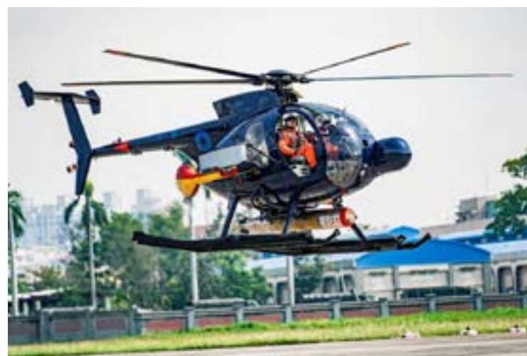
MD-500 of the ROC Navy carrying a single torpedo. ROC Navy picture.
