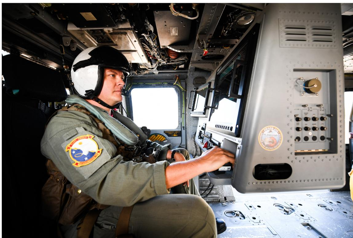
*Naval Aircrewman 1st Class Patrick Miller, assigned to the Dragon Whales of Helicopter Sea Combat Squadron (HSC) 28, operates the common console used for both Airborne Laser Mine Detection System (ALMDS) (pictured) and the Airborne Mine Neutralization System (AMNS) aboard an MH-60S Knight Hawk helicopter. The console controls the ALMDS pod, which collects laser data for initial and requisition minesweeping missions. U.S. Navy photo*
