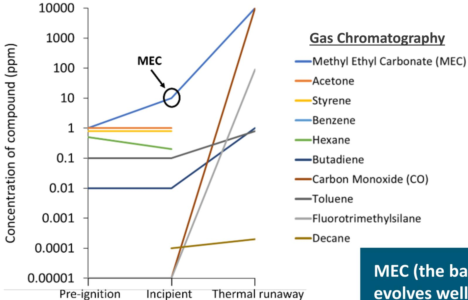
**MEC (the battery electrolyte solvent) evolves well before thermal runaway**
