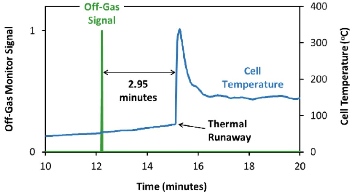
**Overcharge failure test (5C charge rate)
