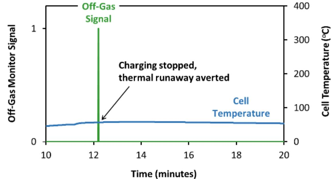
**Overcharge failure test (5C charge rate)
