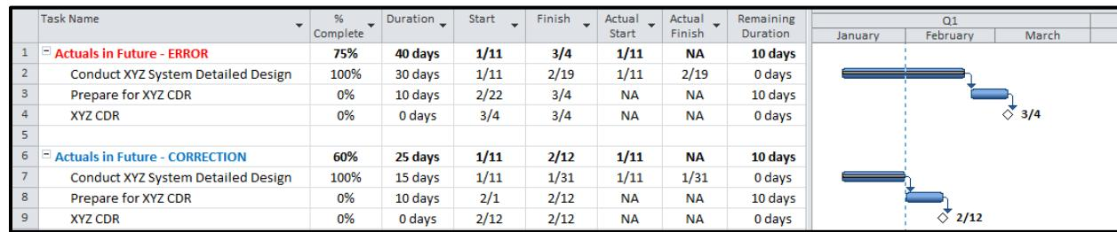
Figure 9.1.1-2 Impact of inaccurate Actual Start to Time Now and the Estimate to Complete (ETC)
