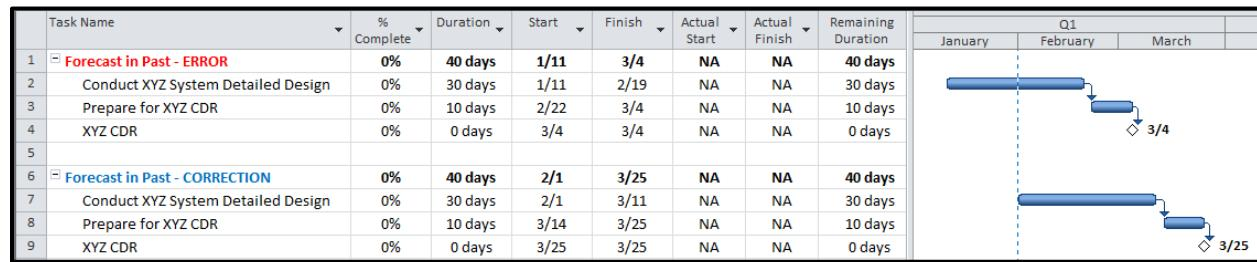
Figure 9.1.1-1 Impact of improper forecast update in the IMS
