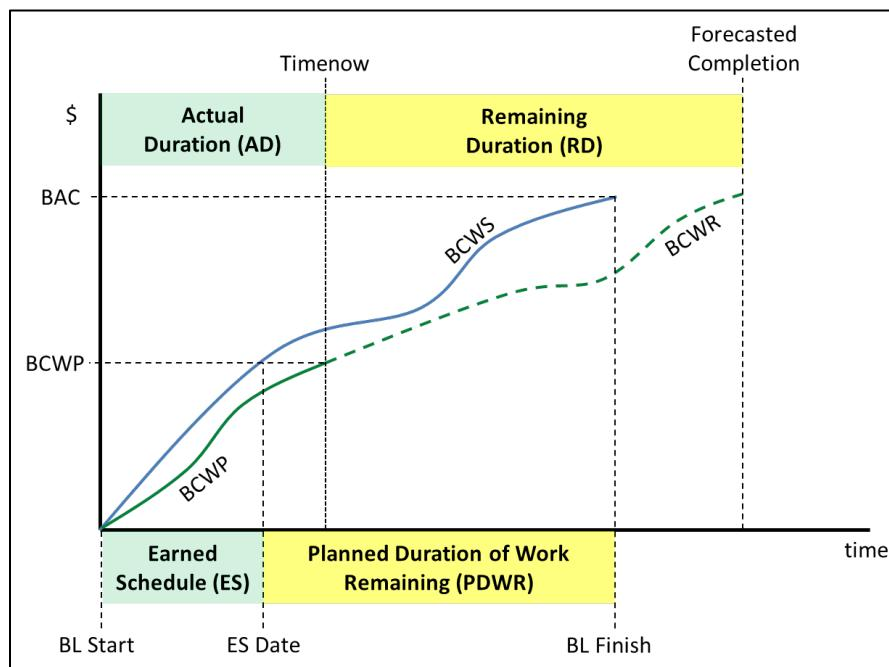
Figure 10.4.10-1 SPI<sub>t</sub> and TSPI<sub>t</sub> calculations
