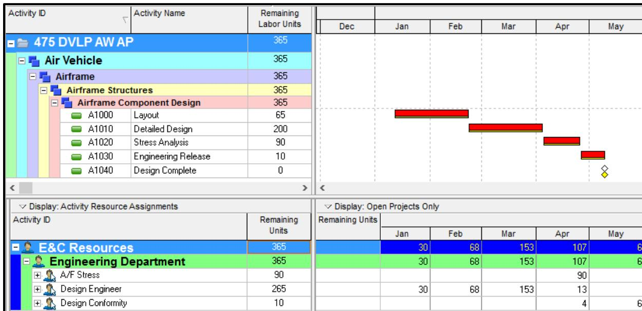
Figure 9.1.4-1 Example of a Resource loaded IMS using Native field resource loading
