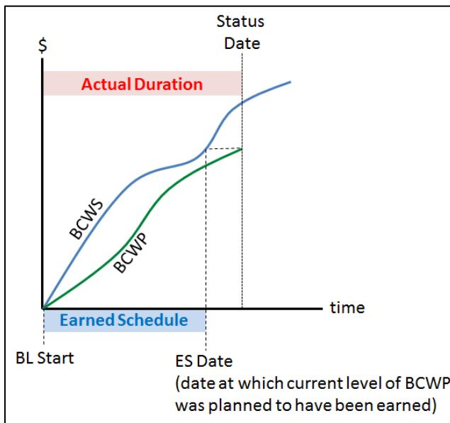
Figure 10.4.9-1 BCWS and BCWP for SPI<sub>t</sub> calculation
