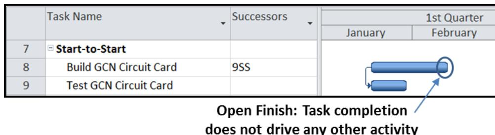
**Figure 5.3-5 Example missing non-Start-to-Start Successor**
