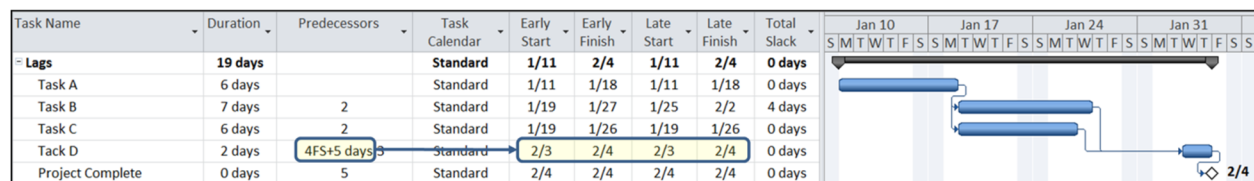
Figure 5.11-4 Example demonstrating the impact a Lag on the Forward and Backward Pass
