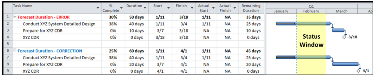
Figure 9.1.2-2 Example of an inaccurate forecast on a task outside of the current Status Window
