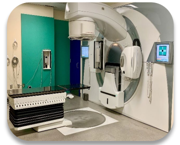
Linear Accelerator Partial body high-energy photon and electron
