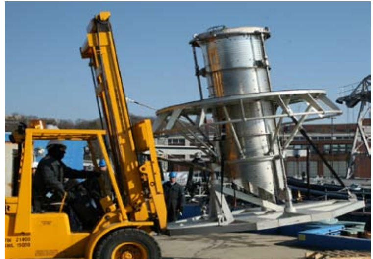
ABOVE RIGHT: TRADITIONAL L&H HARDWARE DESIGN (NOTE EXTENSIVE STAGING AND RIGGING) ABOVE LEFT AND BOTTOM: NEW BEG DIVER PLATFORM DESIGN (DEMONSTRATING EASE OF OPERATION, HANDLING AND TRANSPORTATION)
