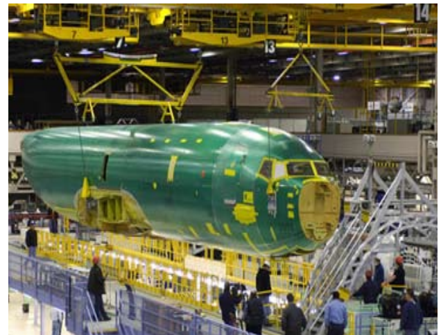
T-1 BEING LOWERED IN THE “JIG” ON 31 MARCH 2008 IN RENTON, WA TO BEGIN FINAL ASSEMBLY
