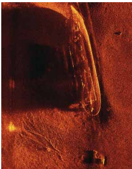
THE SAS-12 SIDESCAN SONAR PRODUCED THIS IMAGE OF A SHIPWRECK. NOTE THE VISIBLE LINES IN THE SAND LEFT BY THE BUOY CHAIN. IMAGE COURTESY OF AUVFEST 2008.
