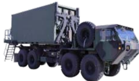
Next Generation Automatic Test System (NGATS) AN/ TSM-191 V6
