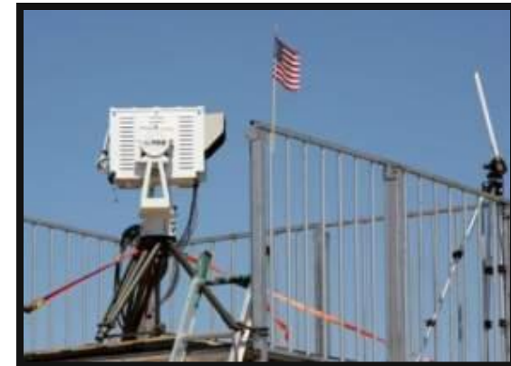
Ground FSO Terminal (courtesy EAGLS program)
