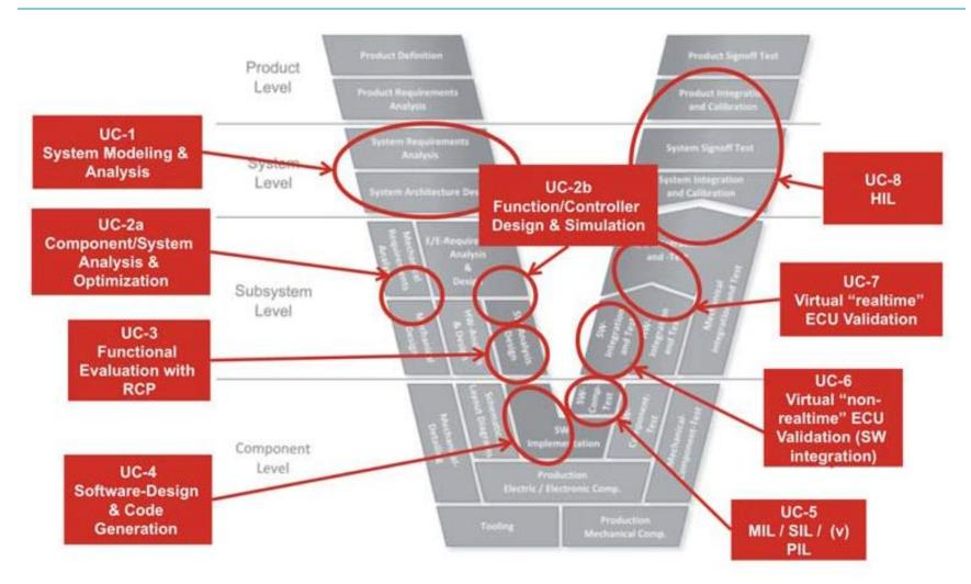
Modification of the V-model in Smart Systems Engineering, Behavior Model Exchange Version 1.0, ProSTEP iViP Recommendation, May 2014
