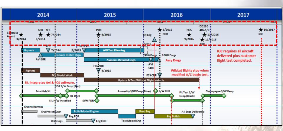
In a purpose built tool the many IMS lines can be coded to fit into a single line on the schedule.
